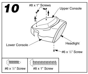
**IMPORTANT!** For packaging reasons, the console/headlight has been pre-assembled at the factory. You will need to disassemble the console/headlight to assemble it to the handlebar.
